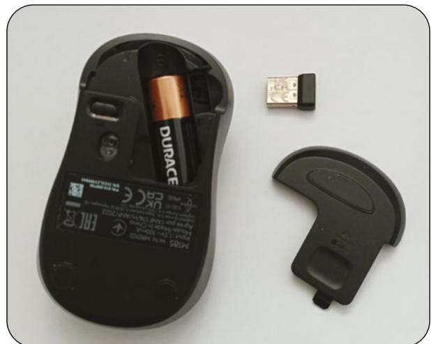
**4** Remove the USB stick and put the slide cover back on.
